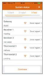
The signal strength is displayed for each connected device. Tap **Issues** to see details of any problems.
