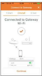
Check that the Gateway is shown as connected to the home Wi-Fi network, and then tap **Continue**
