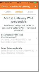
To use the smartphone to get the Gateway serial number automatically, tap Scan gateway QR code
