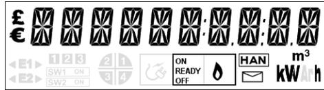
Figure 4: Meter display in 'Test Mode'
