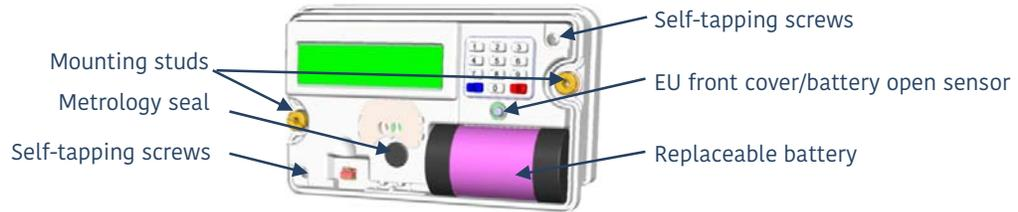
Figure 3: Electronic unit with the cover removed
