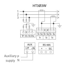
In case of 3Ø3W, VN is replaced by V2 .
