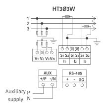
In case of 3Ø3W, VN is replaced by V2.
