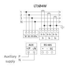
In case of CT/PT operated meter, ensure that meter is connected on secondary side of instrument transformer.
