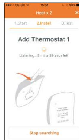
Press and release the button on the top edge of the Thermostat, taking care not to touch the · or ·· buttons on its front face.
