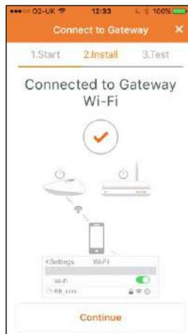
Check that the Gateway is shown as connected to the home Wi-Fi network, and then tap **Continue**
