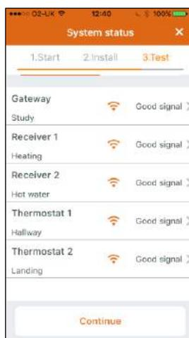
The signal strength is displayed for each connected device. Tap **Issues** to see details of any problems.
