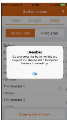
Go to the indicated Thermostat and wake it up by pressing the button on its top edge. It should now display the temperature.
