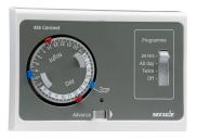
The 425 Coronet timeswitch is a single circuit central heating timeswitch able to switch ON and OFF twice every 24 hours. An advance switch is provided to make temporary overrides to the ON or OFF periods and a selector switch gives a further choice of programmes.
