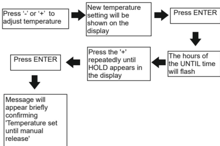
In the 'HOLD' position the temperature can be overridden by pressing either the '-' or '+' buttons. This will then become the new 'HOLD' temperature
