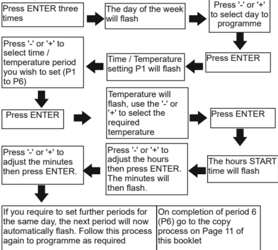
If only two different temperature settings are required in 24 hours then set the first time and temperature using programme one (P1) and the second time and temperature setting using programme setting two (P2). The remaining programmes (P3 to P6) should all be set to the same time and temperature as P2.
