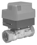
The Z228 valve with changeover auxiliary switch has been designed to control the water circulation in both gravity HW systems and larger fully pumped systems, which employ a single pump by allowing the flow to either or both HW and CH circuits using either a single or separate valves.
