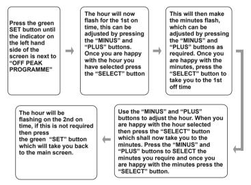
If your electricity tariff offers multiple off peak periods then the 2nd and 3rd off peak periods should be set up by repeating the above procedure. Should you not require any further off-peak settings ensure that the remaining periods are set at the same time. For example; 2nd On 12:00am - 2nd Off 12:00am; 3rd On 12:00am - 3rd Off 12:00am (These are de-fault settings).
